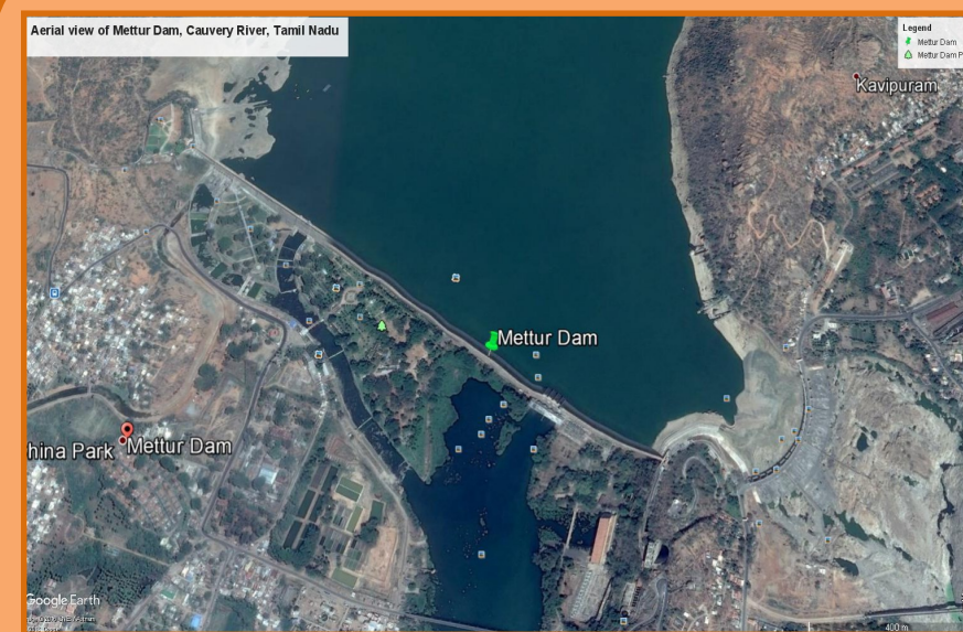
Figure: Aerial view of Mettur Dam, Cauver River, Tamil Nadu. Catchment area is 42217 km 2 , storage capacity is 2708.8 MCM, purpose-irrigation and hydro-electricity. The figure shows the obstructed natural river flow and morphological alteration of the stream
